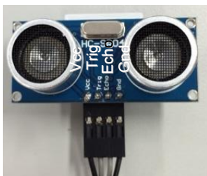
Ultrasonic Sensor The metal side of the female connector should face upward.
